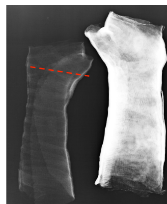
Figure 3. X-ray image of WOODCAST and POP casts.
